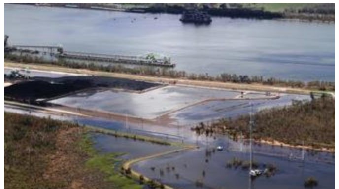
Sept. 2—Floodwaters on and around Kinder Morgan's IMT where containment levees failed, allowing contaminated runoff to escape into the surrounding environment. Photo Credit: Jonathan Henderson, GRN
